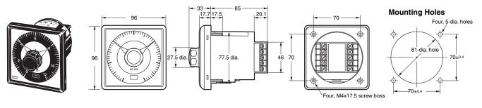
Note: Tightening torque for panel mounting is as follows: 0.3 N·m  $\pm$ 0.05 N·m
