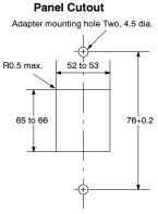
Note: The mounting panel thickness should be 1 to 3.2 mm.
