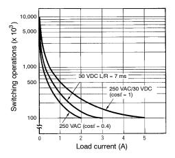
Note: A maximum current of 0.15 A can be switched at 125 VDC (cosf = 1) and a maximum current of 0.1 A can be switched if L/R is 7 ms. In both cases, a life of 100,000 operations can be expected. The minimum applicable load is 10 mA at 5 VDC (failure level: P).
