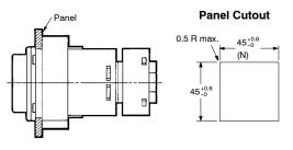
Note: Recommended panel thickness is 1 to 3.2 mm.
