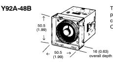
The hard plastic protective cover prevents accidental resetting. It also shields the front panel from dirt and water. The cover is intended for use in areas where unusual service conditions do not exist. The Y92A-48B cover cannot be used with the Y92P Panel Covers below.
