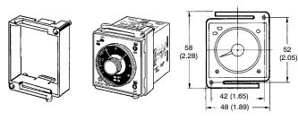
Note: Adapter installs behind the panel. It is ideal for side by side installation. Use P3G-11 or P3G-08 sockets.
