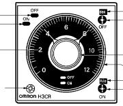
OFF-time unit display window OFF-time unit selector (select one from sec. 10 s, min., and hrs, or from 10 s, 10 min, hrs, and 10 h)
