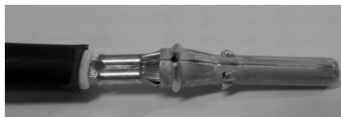
图 4.4.6 定位翅膀(不可被压接) Picture 4.4.6 Locator wings should not be crimped
