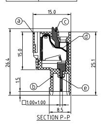
PART NO.: H5 xx 7 0 x 2 00J0 G Color RoHS compliant Solid block 0 Black (RAL9005) (lead<4%) 2 Red (RAL3001/D) No. of poles In copper Alloy 02 2 poles 3 Orange(RAL2011/P) 03 3 poles 4 Yellow(RAL1018/A) 5 Green(RAL6018/T) ... ... 24 24 poles 6 Blue (RAL5015/A) 8 Grey(RAL7035/D) 9 White(RAL1102) C Green(RAL6018/U)
