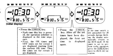
It is also possible to check the timing operations in the sequence they are to be executed. The operations to be performed Thursday are checked. Mode selector switch is in RUN.
