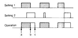
If both settings 1 and 2 are for an ON/OFF or pulse operation, the output is continuously produced without being interrupted. For example, if setting 1 is for cyclic operation, and 2 is set for an ON/OFF operation, the cyclic operation is performed during period of a to b, and the ON/OFF operation is performed from b to c.
