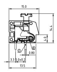
N=Number of poles Dim A=N×5.0+1.5  $Dim B=(N-1)\times 5.0$
