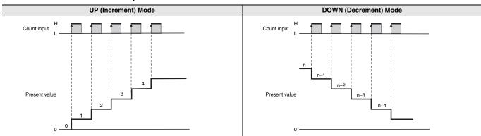
\* Counting starts when the count input is turned ON after turning ON the power.
