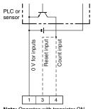
Note: Operates with transistor ON.
