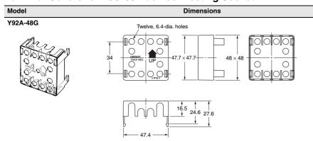
Note: The Terminal Cover can be used with a Back-mounting Socket (P3G-08) to create a finger-safe construction.
