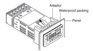
The H8GN's panel surface is water-resistive (conforming to NEMA 4X (indoors) and IP66). In order to prevent the internal circuit from water penetration through the space between the Counter and operating panel, attach a rubber packing (provided with the H8GN) between the Counter and operating panel and secure the rubber packing with the Flush-mounting Adaptor.
