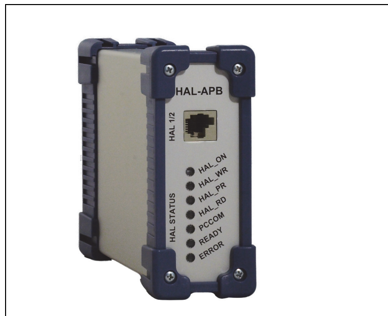
Fig. 1–1: Application Board HAL-APB V1.x
