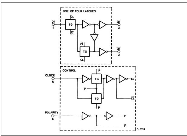
This logic diagram has not be used to estimate propagation delays
