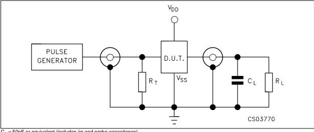
$\begin{array}{l} C_L = 50 \text{pF or equivalent (includes jig and probe capacitance)} \\ R_L = 200 \text{K}\Omega \\ R_T = Z_{\text{OUT}} \text{ of pulse generator (typically 50}\Omega) \end{array}$
