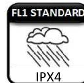
Water Resistant works after splashing water on all sides
