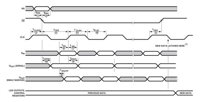
NOTE: 1. DATA IS COPIED TO THE CONTROL REGISTER OR THE DOT LATCH AND LED OUTPUTS WHEN  $\overline{\text{CE}}$  IS HIGH AND CLK IS LOW.
