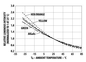
Figure 10. Relative luminous Intensity versus ambient temperature.
