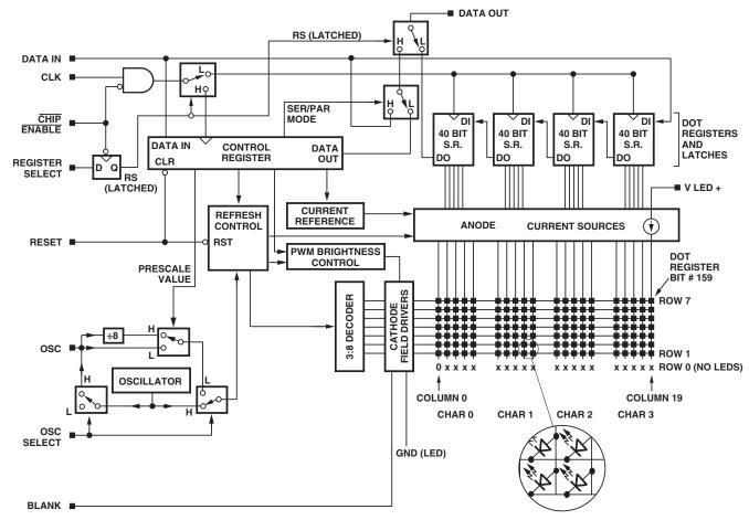
Figure 6. Block diagram for HCMS-39xx.
