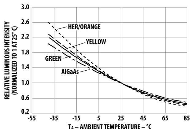
Figure 10. Relative luminous intensity versus ambient temperature.
