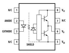
A 0.1  $\mu F$  bypass capacitor must be connected between pins 5 and 8.
