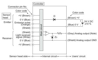
Note: Analog output does not incorporate a short-circuit protection circuit. Do not connect it directly to a power supply or a capacity load.
