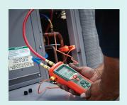
Extech's Heavy duty Digital Manifold/Pressure Gauge simultaneously measures suction line or liquid line pressure and line temperature to calculate and display superheat and sub cooling for A/C units. It also has dual inputs measuring differential pressure (P1-P2) and Type K temperature (T1-T2). For use with R22 and R410A refrigerants. Included are heavy duty connection hoses, Type K Temperature Clamp probe, and bead wire Temperature probe.
