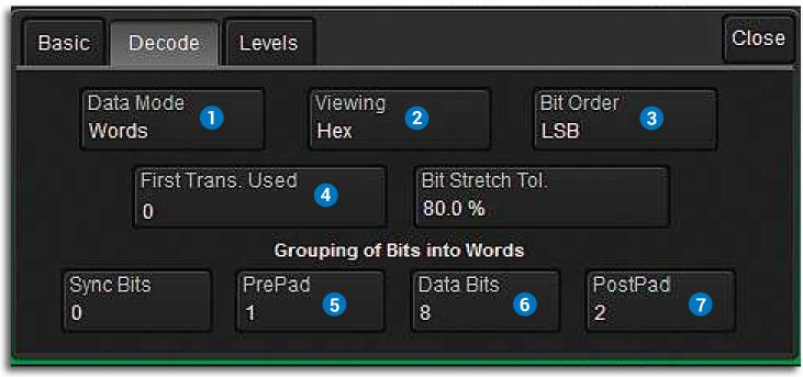
User-definable protocol controls enable flexible serial bus decoding.
