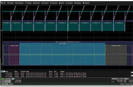
Quickly decode serial buses that use Manchester and NRZ encoding schemes with configurable, user-definable protocol formats.
