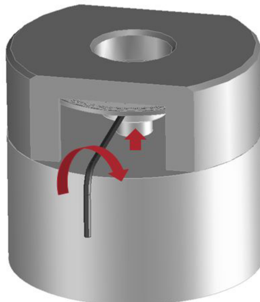
Figure 1d. Tighten the set screws
