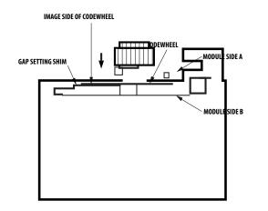
Figure 2. Alignment Tool is Used to Set Height of Codewheel.
