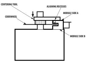
Figure 3. Alignment Tool is Placed over Shaft and onto Codewheel Hub. Alignment Tool Pins Mate with Aligning Recesses on Module.
