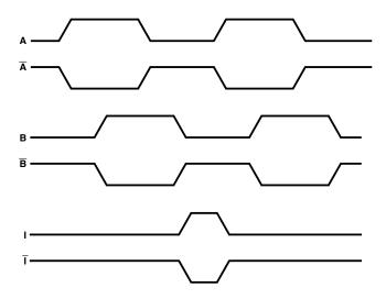
Waveforms for Encoders with Line Drivers.
