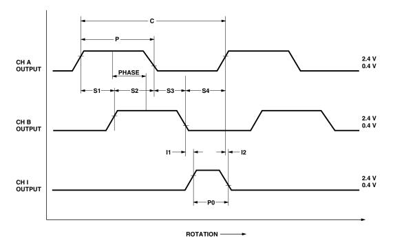
Waveforms for Encoders without Line Drivers.
