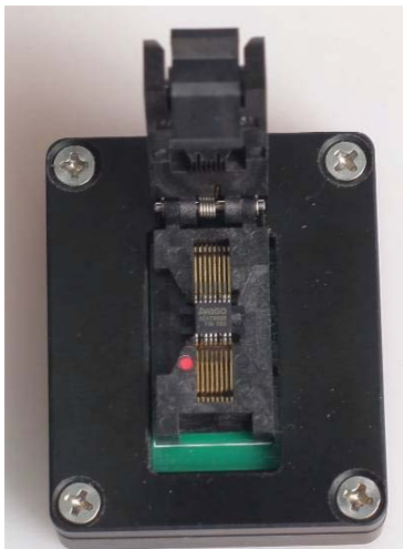
Figure 25. Ensure pin 1 of the encoder IC is aligned with the red dot
