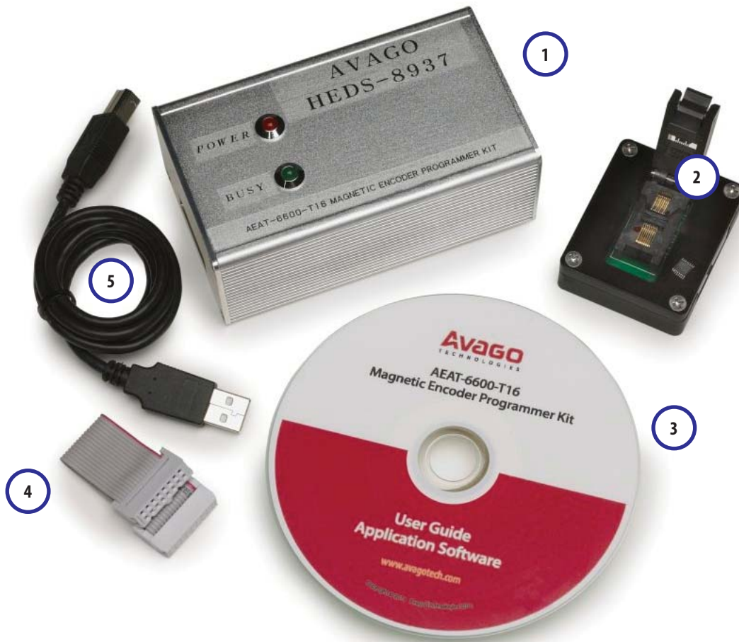
Figure 2. Components of the programmer kit
