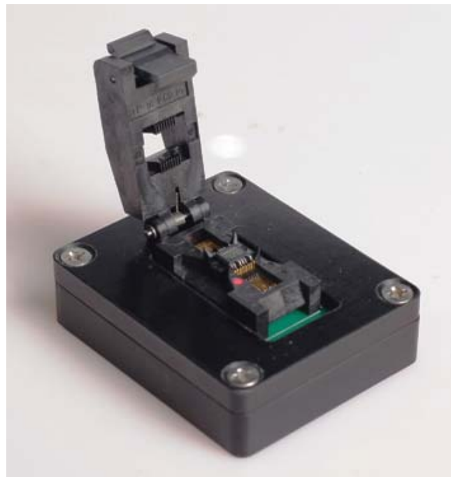
Figure 5. The IC adapter socket has a red dot that indicates pin 1 of the AEAT-6600-T16 encoder
