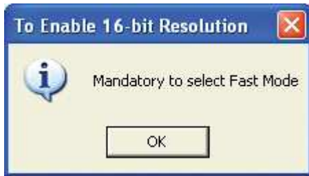
Figure 14. Pop up message for mandatory incremental setting when selecting 16-bit for absolute.
