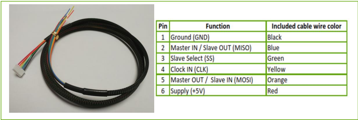
Figure 4 Cable Pin Configuration
