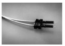
Manually press connectors together in the center of the arrangement. Then latch by pressing on the sides of each connector. As with the simplex version, connectors are secured when top halves latch into the ferrule halves.
