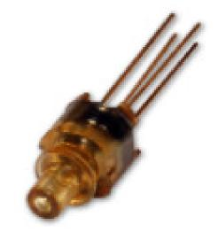
The HFD3180-103 use a high-performance GaAs PIN photo-detector packaged with a transimpedance amplifier designed to meet performance requirements for data rates up to 2.5Gbps data communication over multi-mode optical fiber at 850nm. Applications include Ethernet, Fiber Channel and ATM protocols. The optical assembly is designed to interface either 50mm or 62.5mm multi-mode fiber.
