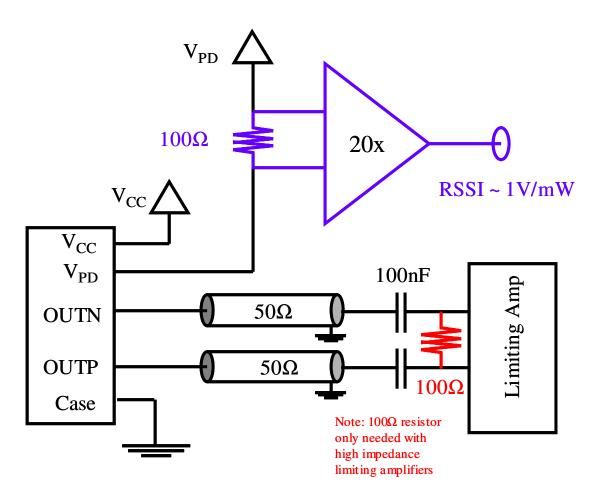
Optional RSSI implementation is shown in blue, implemented on HFD3180-103 only Optional  $100\Omega$  differential termination for high impedance limiting amplifiers is shown in red.
