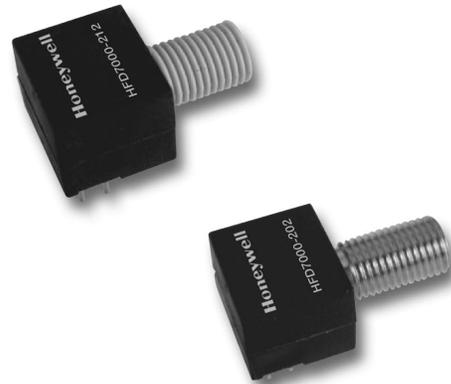
The HFD7000 Series are high-speed optical receivers designed for data transmission in industrial LAN applications. The monolithic CMOS chip consists of a large area photodiode, pre-amplifier with controlled gain, a post amplifier, a comparator and TTL output stage. The integrated voltage regulator provides easy use in many applications.
