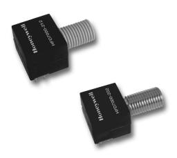
The HFD7000 Series are high-speed optical receivers designed for data transmission in industrial LAN applications. The monolithic CMOS chip consists of a large area photodiode, pre-amplifier with controlled gain, a post amplifier, a comparator and TTL output stage. The integrated voltage regulator provides easy use in many applications.
