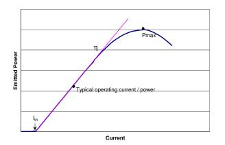
Emitted Power vs. Current: Power varies approximately Threshold Current vs. Temperature: Threshold current varies parabolically with temperature; thus it can be nearly constant for a limited temperature range.
