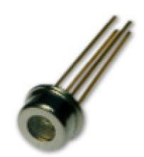
These products are high-performance 850nm VCSELs (Vertical Cavity Surface-Emitting Lasers) designed for high-speed data communications and packaged with a custom designed power monitor diode. The power monitor diode can be used with appropriate feedback control circuitry to set a maximum power level for the VCSEL. These combined features simplify design for high data rate communication and eye safety.
