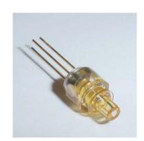
This product is a high-performance 850nm VCSELs (Vertical Cavity Surface-Emitting Lasers) designed for high-speed data communications and packaged with a custom designed power monitor diode. The power monitor diode can be used with appropriate feedback control circuitry to set a maximum power level for the VCSEL. These combined features simplify design for high data rate communication and eye safety.
