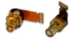
The HFE6x92-761 uses a high-performance Vertical Cavity Surface Emitting Laser (VCSEL) designed to meet performance requirements for 10Gbps data communication over multimode optical fiber. Applications include Ethernet, Fibre Channel and ATM protocols. The optical assembly is designed to inter-face either 50 m or 62.5 m multimode fiber and ensure launch conditioning requirements compatibility with enhanced bandwidth fiber as specified by TIA 455-203.
