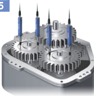
Transmission parts height measurement
