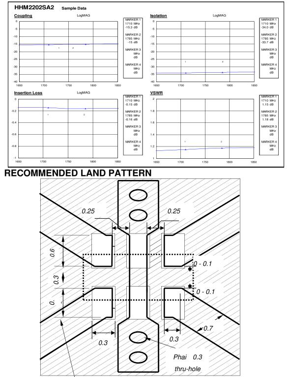
This width is 50ohm. Micro-strip line for 0.4mm thick glass-epoxy substrate.
