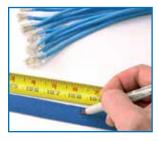
Measure the sleeving to length. Keep the sleeving relaxed and don't pull it as you measure. The most accurate method is to measure the sleeving on the actual application. There will be some foreshortening of the sleeving as it expands over large bundles or connectors. Mark the cut line with a pen or marker.
