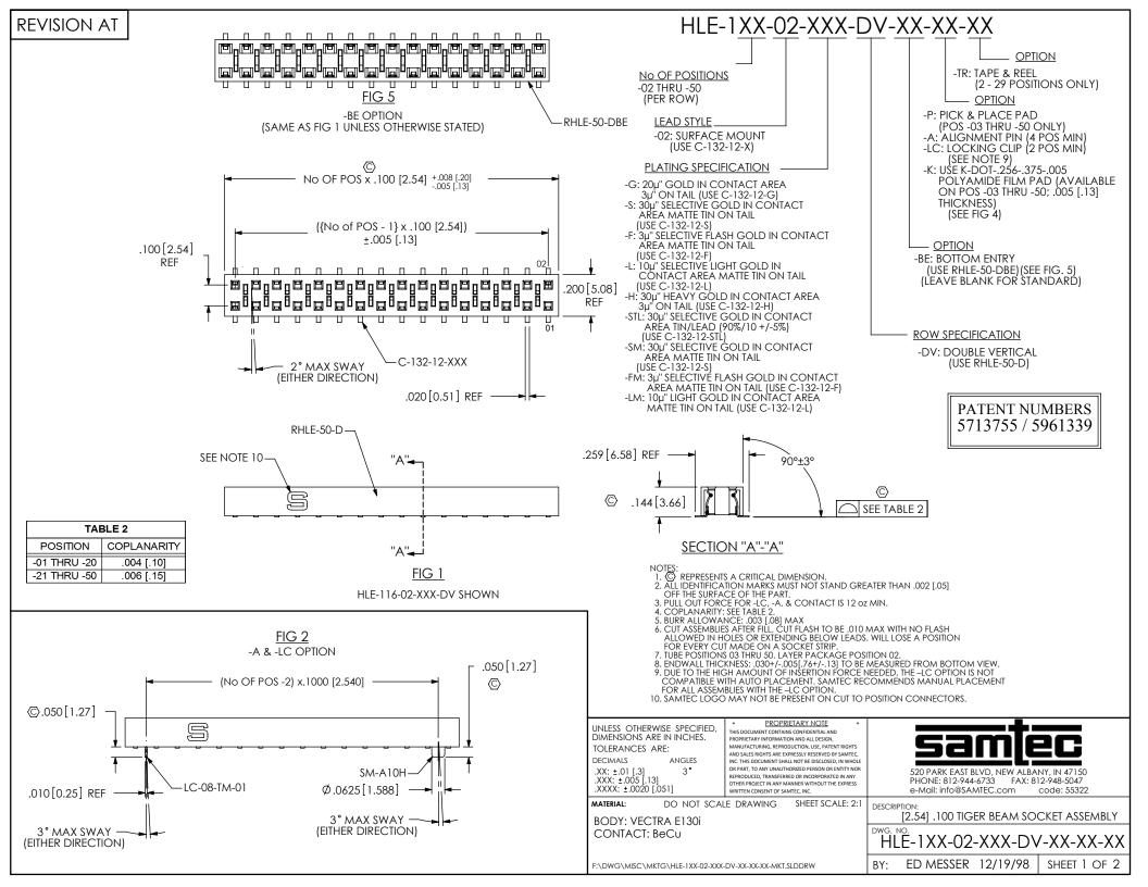
FIG 3 (-P: PICK AND PLACE PAD) AVAILABLE ON POSITIONS 03 THRU 50
