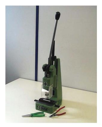
Figure 17 -- Connector Removal tooling HM2Y350
