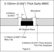
**General Handling:** Handle the chip along the edges with a vacuum collet or with a sharp pair of bent tweezers. The surface of the chip has fragile air bridges and should not be touched with vacuum collet, tweezers, or fingers.
