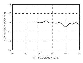
Note: Measured Performance Characteristics (T<sub>OP</sub> = 25°C)
