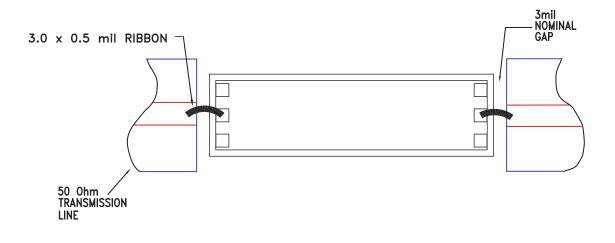
Note 1: Best performance obtained from use of <10 mil (long) by 3 by 0.5 mil ribbons on input and output.
