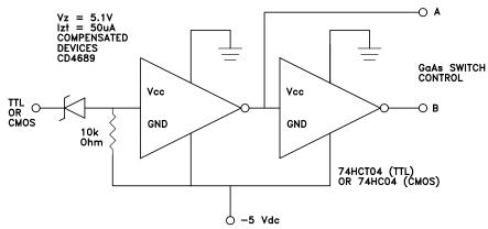
Simple driver using inexpensive standard logic ICs provides fast switching using minimum DC current while translating from standard positive voltage TTL or CMOS logic to negative voltage GaAs IC logic.
