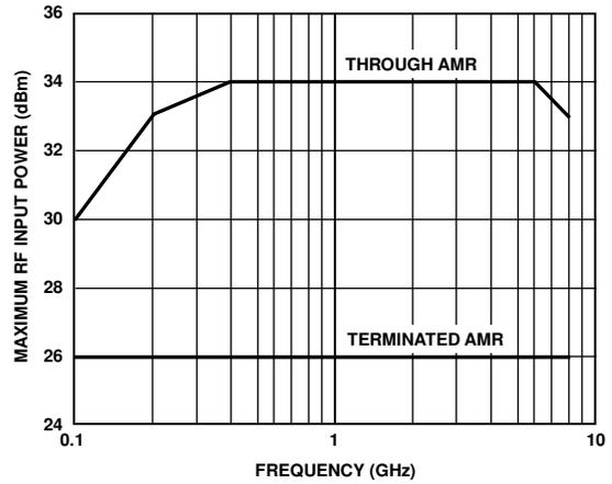
Figure 2. Maximum RF Input Power vs. Frequency
