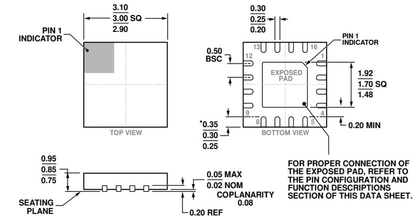
\*COMPLIANT WITH JEDEC STANDARDS MO-220-VEED-4 WITH THE EXCEPTION OF PACKAGE EDGE TO LEAD EDGE.
