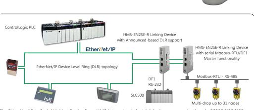
The EtherNet/IP to Serial Linking Device from HMS integrates industrial devices communicating via RS232/422/485, Modbus RTU and DF1 with a Rockwell PLC. You do all configuration in your familar Rockwell Studio 5000 environment.
