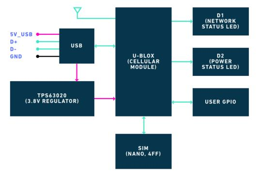
Below is the block diagram for the u-blox SARA-U201 module.
