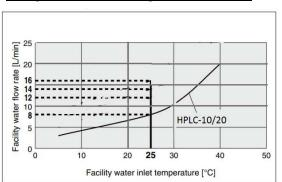
\* This is the facility water flow rate at the circulating fluid rated flow rate and the cooling capacity listed in the "Cooling Capacity" specifications.
