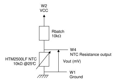
$$V_{OUT}(mV) = \frac{V_{CC}(mV) * NTC_{HTM2500LF}(\Omega)}{R_{batch}(\Omega) + NTC_{HTM2500LF}(\Omega)}$$
