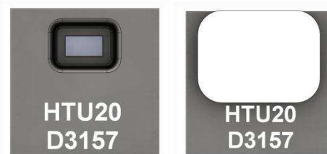
Laser marking on HTU20D(F) sensor
