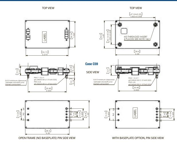
$\odot\,$  M3 bolts must not exceed 0.138 ''(3.5mm) depth below the baseplate surface. @ Applied screw torque must not exceed 5.3 in-lb. (0.6 N-m).
