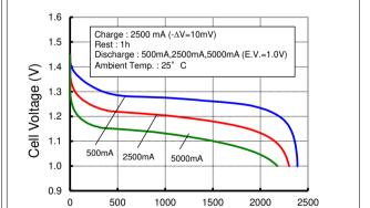
Discharge Capacity (mAh)
