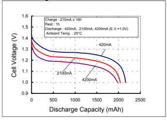
Charge: 210mA×16h, Discharge: 420mA(E.V.=1.0V) at 20°C
