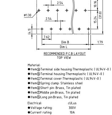
Wire range: •Solid wire(AWG): 12-28 •Stranded wire(AWG): 12-28 •Wire strip length: 5-6mm Withstanding Voltage: 1.6KV •Operating temperature: -40°C to +115°C 260°C±5°C/5 Sec •Soldering temperature:
